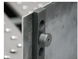
Magnet keeps sheet metal in vertical position
