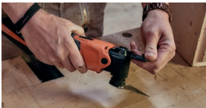
To release the blade, lift the locking lever...
